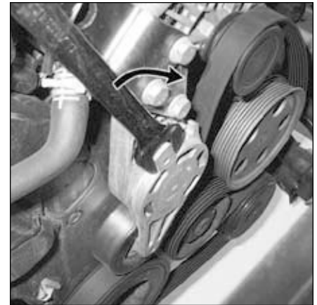
19.6 Rotate the tensioner arm to relieve belt tension
