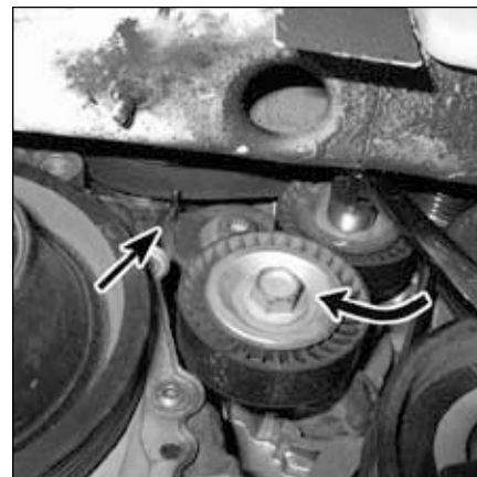
19.14 Rotate the tensioner clockwise, then insert a drill bit to lock the tensioner body
