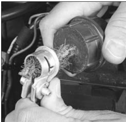
11.7b When cleaning the cable clamps, all corrosion must be removed (the inside of the clamp is tapered to match the taper on the post, so don't remove too much material)
