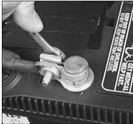
11.6 Use a wrench to check the tightness of the battery cable bolts when removing corroded bolts, special battery pliers may be needed
