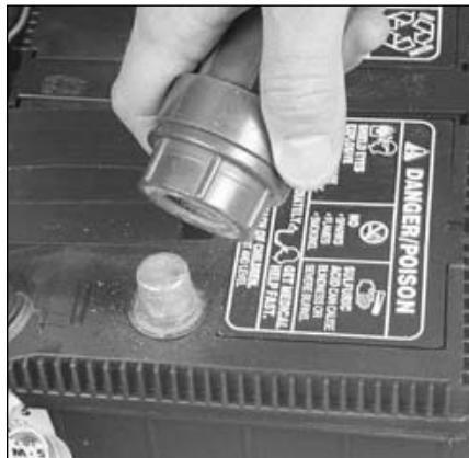
11.7c Regardless of the type of tool used to clean the battery posts, a clean, shiny surface should be the result
