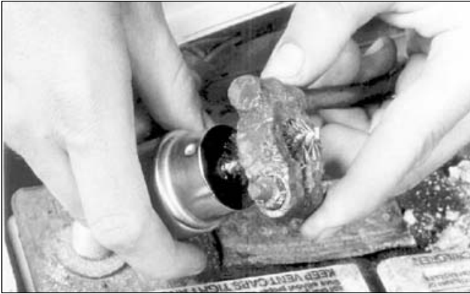
11.7a When cleaning the cable clamps, all corrosion must be removed (the inside of the clamp is tapered to match the taper on the post, so don't remove too much material)
