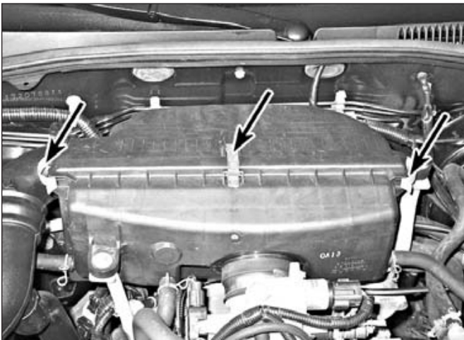
17.1a Release the spring clips to access the filter element (early models)
