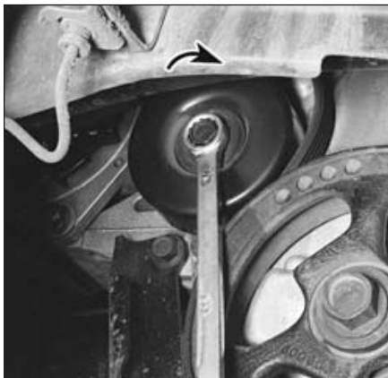
11.4 Use a 14 mm wrench to lift the tensioner in the direction shown to release the tension from the belt
