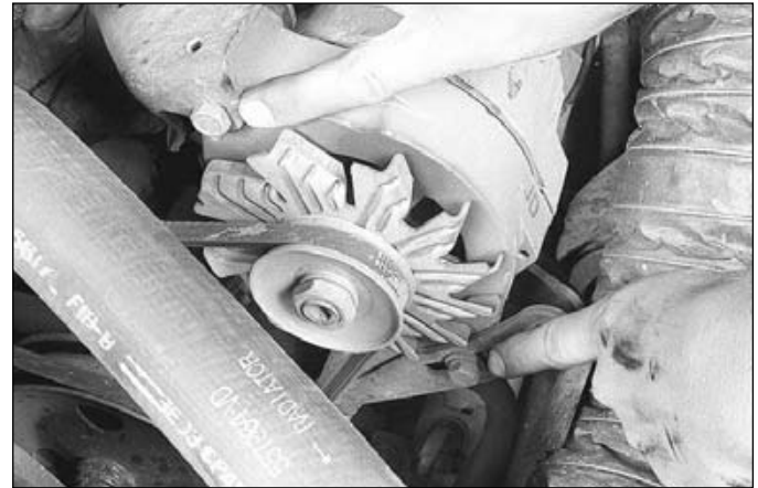
9.6 Nearly all belt-driven components have a pivot bolt (top) and a strap or adjusting bolt (near bottom of alternator shown)
