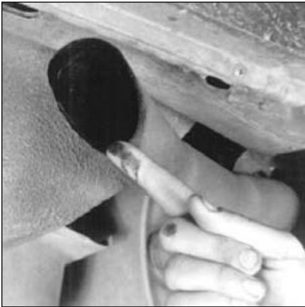
7.5 Black, sooty deposits at the end of the exhaust pipe may be an indication that the carburetor needs adjustment or the engine is in need of a tune-up
