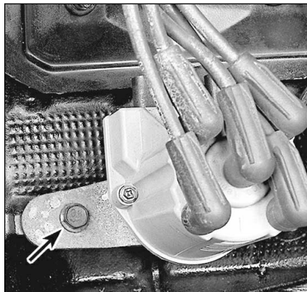
38.14 The distributor hold-down bolt (arrow) should be loosened just enough to rotate the distributor slightly
