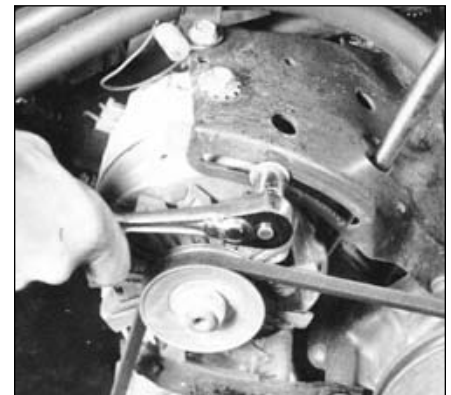
27.8 Adjust the belt tension by gently prying on the component as the adjustment bolt is tightened
