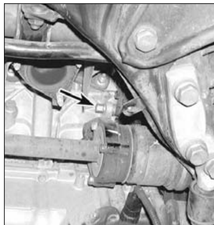
12.5b From below, loosen the bolt (arrow) at the back of the power steering pump . . .
