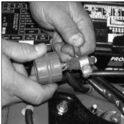
10.7a When cleaning the cable clamps, all corrosion must be removed (the inside of the clamp is tapered to match the taper on the post, so don't remove too much material)
