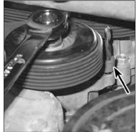
11.7 Release the tension using a wrench, then insert a drill bit or rod to lock the tensioner in place (four-cylinder engine)
