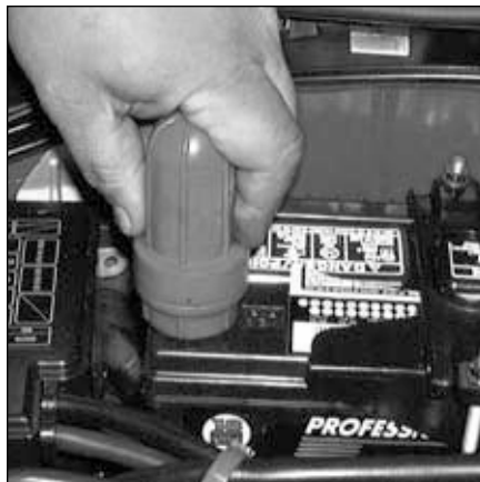
10.7b Regardless of the type of tool used to clean the battery posts, a clean, shiny surface should be the result
