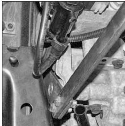
18.9c Locate the tool over the tensioner arm pivot bolt head . . .
