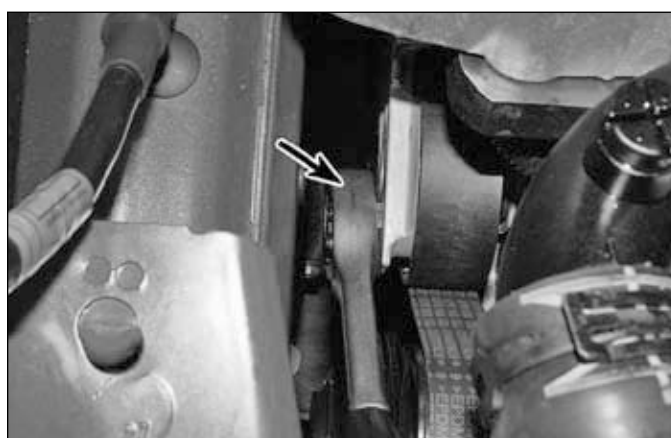
18.5a Engage a 3/8-inch drive ratchet with the square hole in the drivebelt tensioner arm
