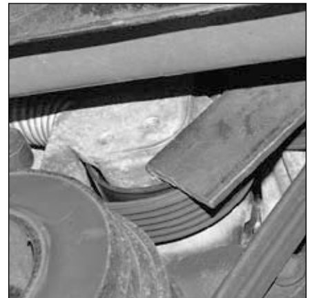
18.9d . . . ensure the lower end of the tool doesn't slip from the bottom of the arm
