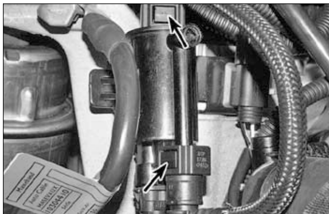
18.1 Press-in the buttons to disconnect the hoses from the tank vent valve
