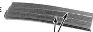
13.3b Small cracks in the underside of a V-ribbed belt are acceptable - lengthwise cracks, or missing pieces that cause the belt to make noise, are cause for replacement
