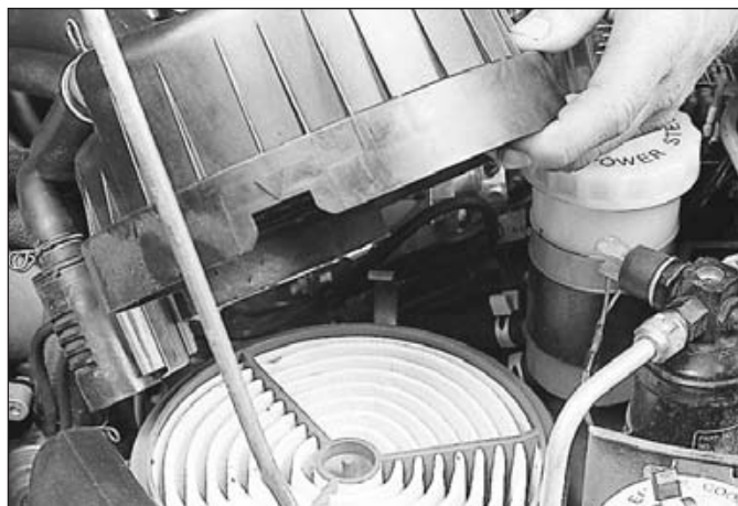
29.9 With the hoses still attached, pull the cover up, then lift the element out of the housing
