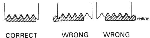
11.10 When installing the V-ribbed belt, make sure it is centered on the pulley - it must not overlap either edge of the pulley
