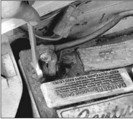
10.6b Removing the cable from a battery post with a wrench - sometimes special battery pliers are required for this procedure if corrosion has caused deterioration of the nut hex (always remove the ground cable first and hook it up last!)
