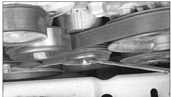
24.7 Rotate the tensioner arm to relieve belt tension (3.0L engine shown, 3.8L engine similar)
