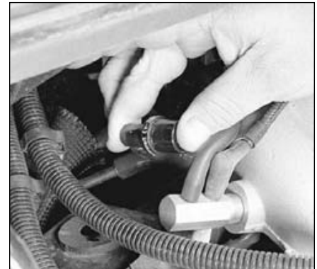
25.2 With the engine running at idle, remove the PCV valve and verify that vacuum can be felt at the end of the valve
