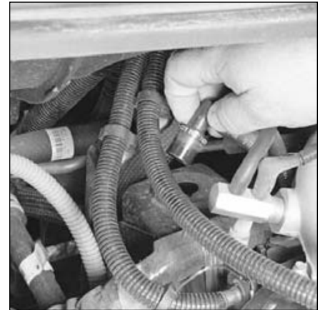
25.1 The PCV valve on 3.0L engines is located in the right (rear) valve cover and on 3.8L engines in the left (front) valve cover
