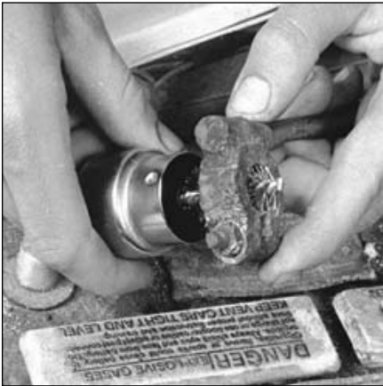
20.5d Cleaning the battery cable clamp with the special tool
