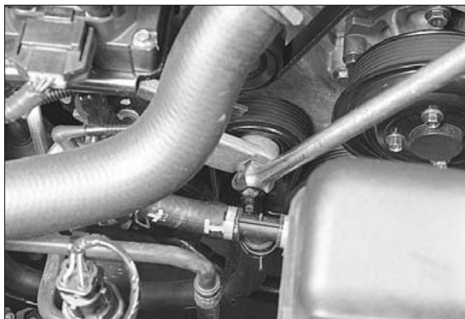
29.6 Rotate the tensioner arm to relieve belt tension
