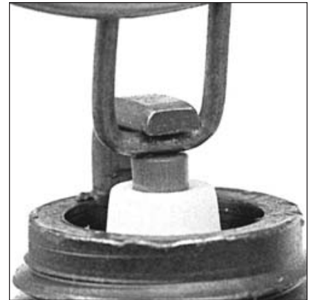
31.5a Spark plug manufacturers recommend using a wire-type gauge when checking the gap - if the wire does not slide between the electrodes with a slight drag, adjustment is required
