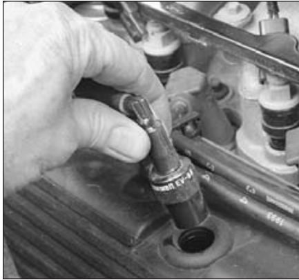
30.2 With the engine running at idle, remove the PCV valve and verify that vacuum can be felt at the end of the valve
