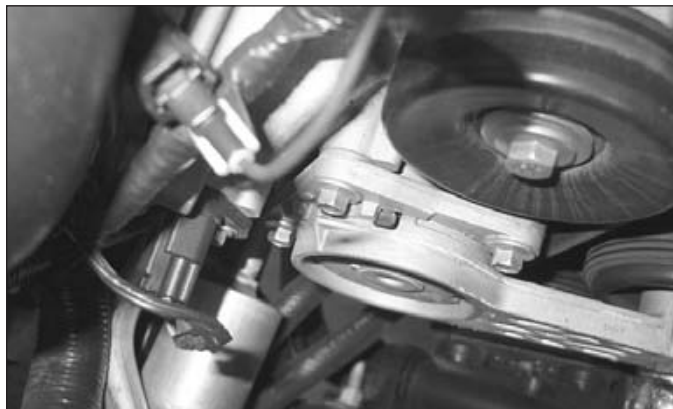
21.5 Belt wear indicator marks are located on the side of the tensioner body - when the belt reaches the maximum wear mark it must be replaced
