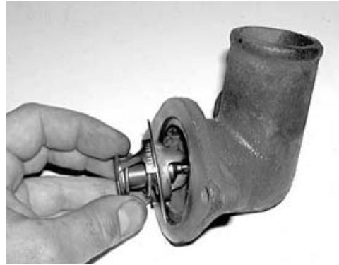
Fig.2.1 Correct location of thermostat (Sec. 6)
