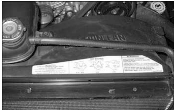
19.8 The routing schematic for the serpentine belt is usually found on the fan shroud
