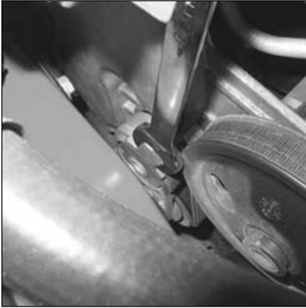
19.8 Use an open end wrench to rotate the drivebelt tensioner clockwise to release tension on the belt
