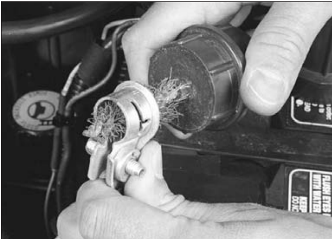
11.7a When cleaning the cable clamps, all corrosion must be removed (the inside of the clamp is tapered to match the taper on the post, so don't remove too much material)
