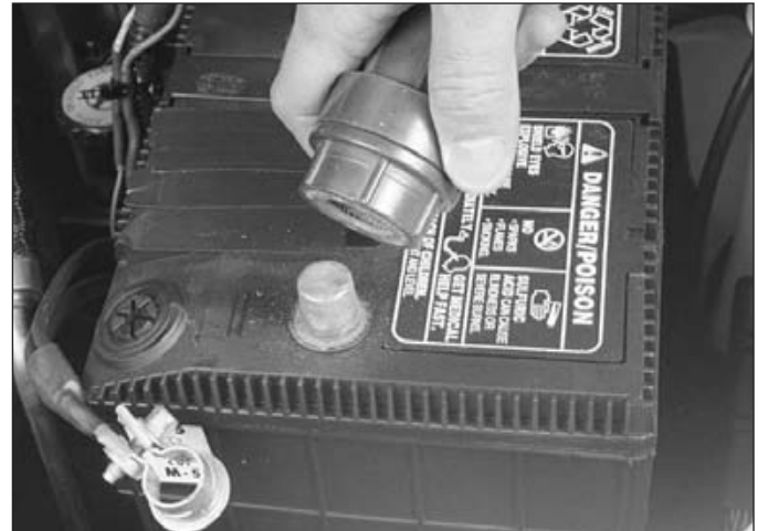
11.7b Regardless of the type of tool used on the battery posts, a clean, shiny surface should be the result
