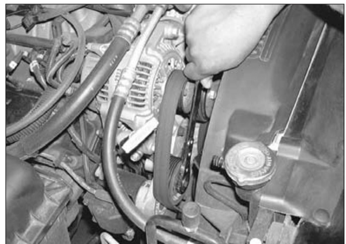
12.6 Rotate the automatic tensioner (V6 and V8) by turning its center bolt clockwise with a long wrench until the belt can be pulled off the pulley, then release the tensioner
