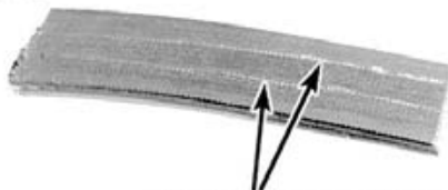
Cracks Running Parallel to "V" Portions of Belt
