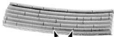
Cracks Running Across "V" Portions of Belt
