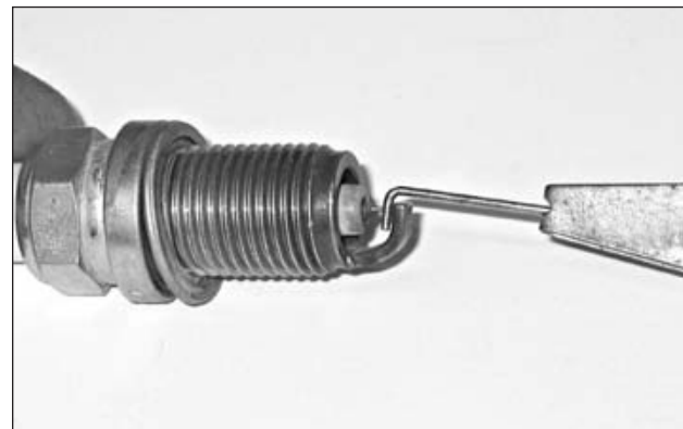
21.5 Spark plug manufacturers recommend using a wire-type gauge when checking the gap - the wire should slide between the electrodes with a slight drag
