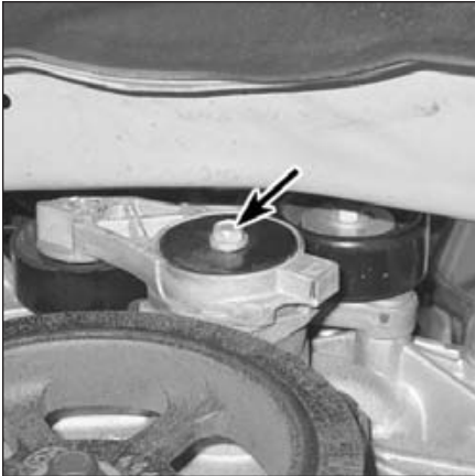
19.18 The drivebelt tensioner is secured by a single bolt
