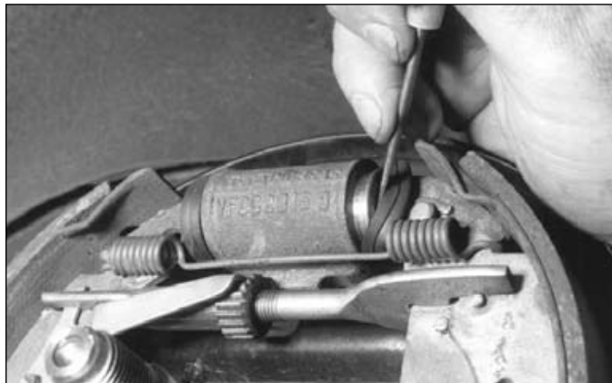
18.16 Use a small screwdriver to carefully pry the boot away from the cylinder and check for fluid leakage
