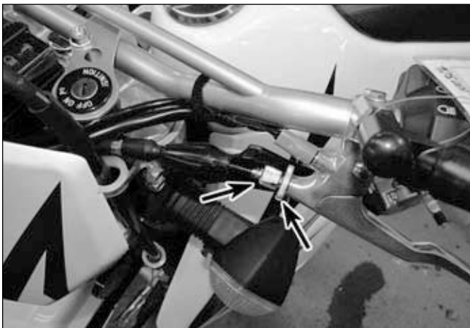
19.3b Loosen the locknut (right arrow) and turn the adjuster (left arrow) to adjust the cable
