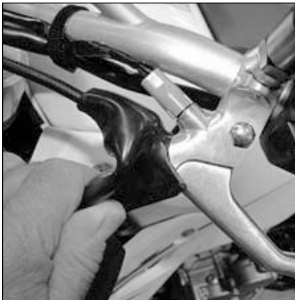
19.3a Pull the rubber boot back from the adjuster
