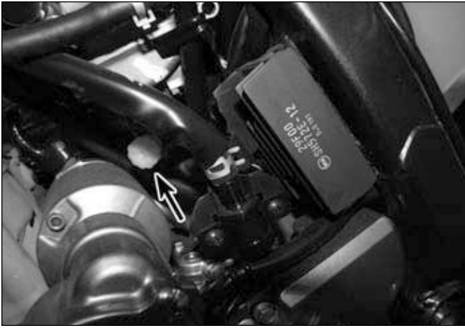
20.3 Adjust the idle speed with the throttle stop screw
