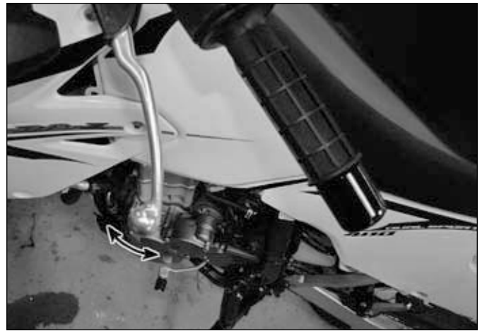
19.2 Measure clutch lever freeplay at the lever tip
