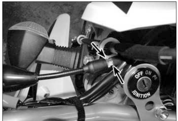
19.4 Make major cable adjustments at the inline adjuster - loosen the locknut (left arrow) and turn the adjuster (right arrow)
