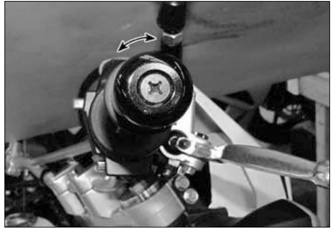
21.3 Check throttle lever freeplay at the lever tip
