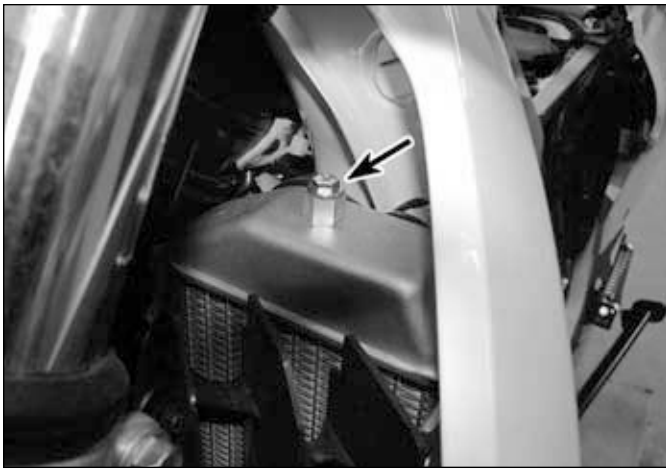
18.24 The cooling system air bleed bolt is located in the top of the left-hand radiator
