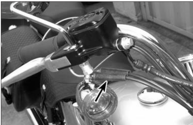
10.3a Pull back the rubber covers from the throttle cable adjusters (arrow) . . .
