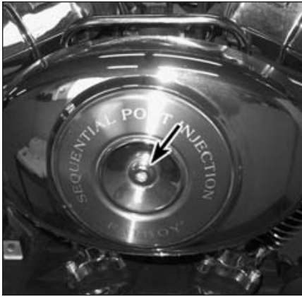
9.1 Remove the center screw and take off the air cleaner cover . . .
