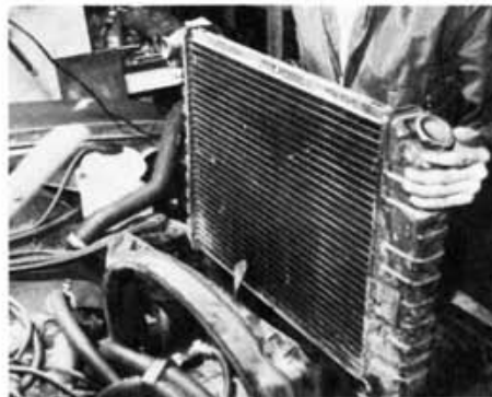
5.6 Removing the radiator. The shroud is
