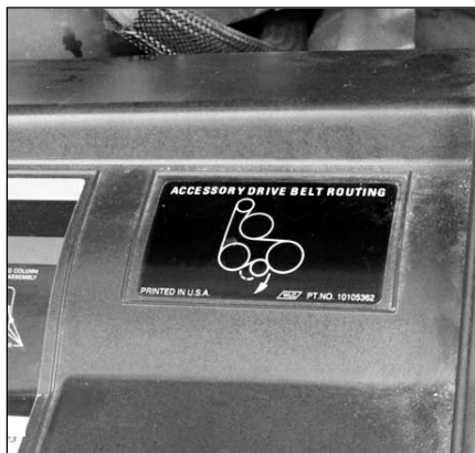
26.7 On most models, the serpentine drivebelt routing diagram is located on the radiator support
