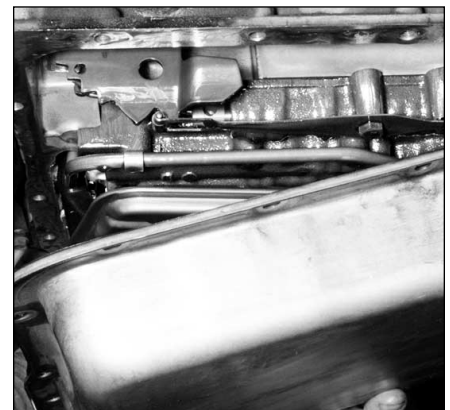
27.6 With the rear bolts in place but loose, pull the front of the pan down to drain the transmission fluid
