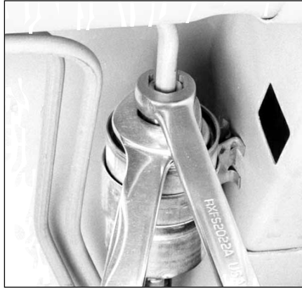
25.3e Use one wrench to steady the filter, then unscrew the fuel line fitting and remove the filter (if available, use a flare nut wrench on the fuel line fitting)
