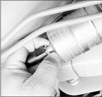
25.3d Depress the white plastic quick-disconnect tabs and detach the fuel lines from the filter - wrap a rag around the fuel line to absorb the fuel that will run out
