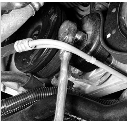
26.5 Rotate the tensioner clockwise to remove or install the belt
