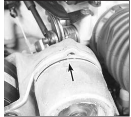
6.3 The arrow on the tensioner must be within the marked range - if it isn't, the belt is stretched and must be replaced
