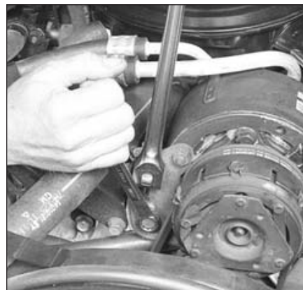
6.9 Use a 1/2-inch drive breaker bar in the square hole provided, to tension the air conditioning compressor drivebelt
