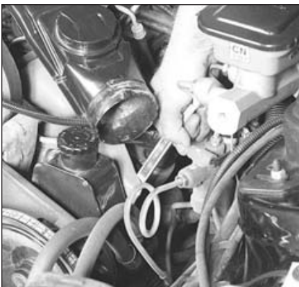
6.7b One of the power steering pump adjustment bolts is located behind the pump
