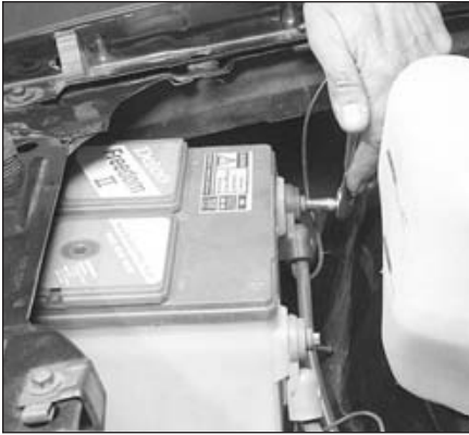
5.3 Unlike older model batteries, the cable terminals are on the side of these batteries
