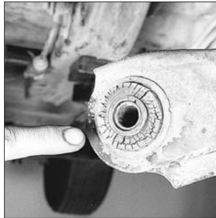
8.6 Rubber bushings in the steering and suspension systems will deteriorate and crack after a time, indicating replacement is necessary
