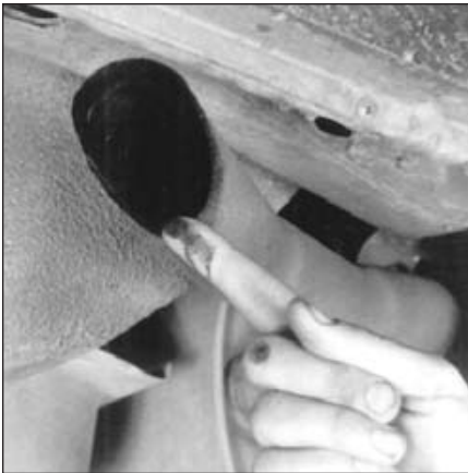
8.5 Black, sooty deposits at the end of the exhaust pipe may be an indication that the carburetor needs adjustment or the engine is in need of a tune-up
