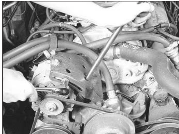
9.6 Nearly all belt-driven components have a pivot bolt (top) and a strap or adjusting bolt (near bottom of alternator shown)
