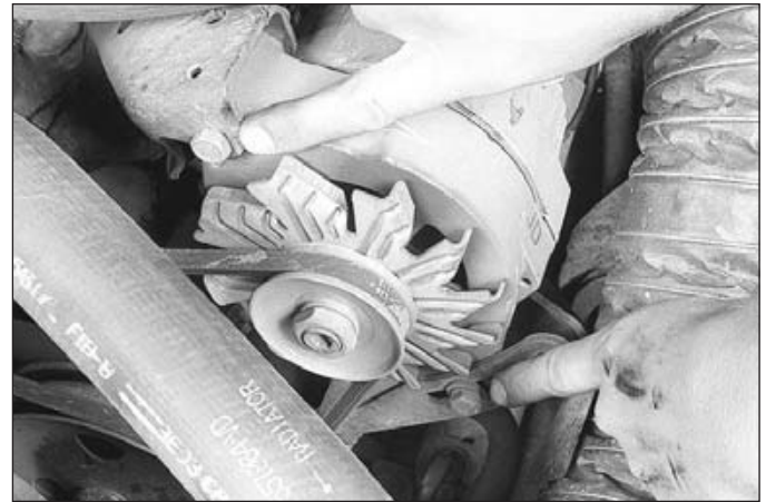
9.6 Nearly all belt-driven components have a pivot bolt (top) and a strap or adjusting bolt (near bottom of alternator shown)
