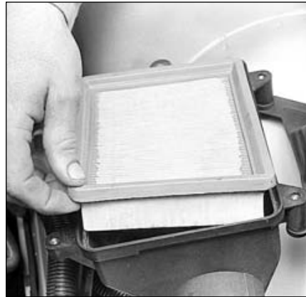
20.2b . . . then pull the air filter element out of the housing
