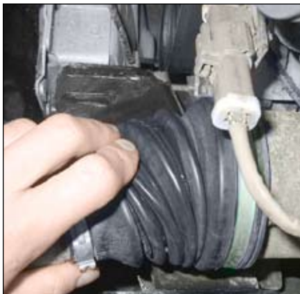
19.2 Flex the driveaxle boots by hand to check for cracks and/or leaking grease
