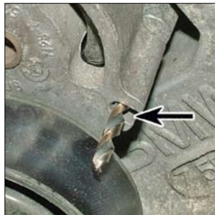
20.7 Insert a rod or drill bit into the holes to lock the tensioner in the compressed position
