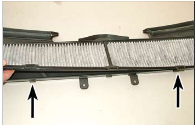
18.3 Release the clips and lift out the cabin air filter element
