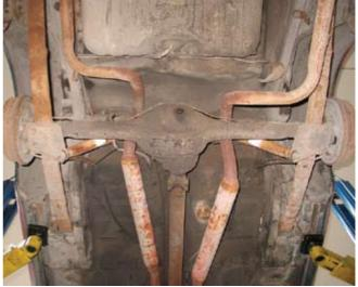
**4a.16** Our exhaust system was composed of incorrect muffler-shop pipes and a pair of cheap glasspack mufflers welded in place. We will be using new, correct exhaust pipes for our car, with the OEM-style mufflers for factory single-exhaust as original on a base V8 like ours. The easiest way to remove our all-welded system was to cut it into sections with a reciprocating saw.
