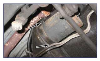
**4a.13** Disconnect the electrical connectors at the starter motor, then remove the two starter mounting bolts and remove the starter. \*\*Warning: Make sure the battery has been removed from the vehicle (or at least disconnected) before doing this.
