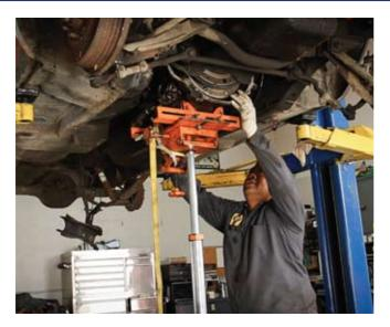
**4a.15** Roll the transmission jack rearward and slowly lower it to the floor. The transmission should be secured to the jack with hooks and chains (or a strap as is being used here).
