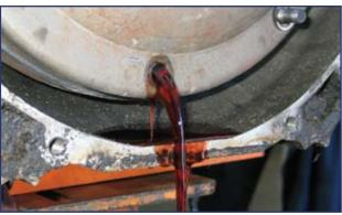
**4a.14** Support the back of the engine to the body with a chain, then gently separate the transmission from the engine and move it rearward enough to access the two converter drain plugs to drain the fluid from the converter. Such a convenient way to drain the converter is one of the perks of working on older cars. Modern cars don't have converter drain plugs.
