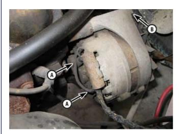
**4a.19** Disconnect any ground wires from the engine to the chassis. Disconnect the wires at the alternator (A), remove the alternator adjuster and mounting bolts (B), and remove the alternator.
