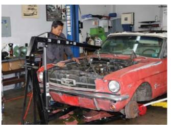
**4a.20** Remove the battery (if not already done) and air filter housing, then attach chains to the front and rear of the engine to begin engine removal. Drain the oil and remove the oil filter, if not already done.
