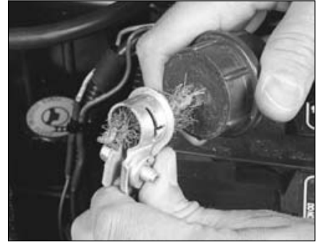
11.7a When cleaning the cable clamps, all corrosion must be removed (the inside of the clamp is tapered to match the taper on the post, so don't remove too much material)
