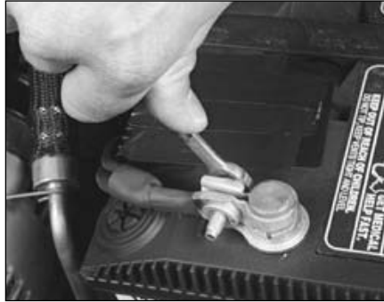
11.6b Removing a cable from the battery post with a wrench - sometimes a special battery pliers is required for this procedure if corrosion has caused deterioration of the nut hex (always remove the ground cable first and hook it up last!)
