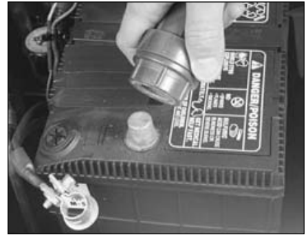
11.7b Regardless of the type of tool used to clean the battery posts, a clean, shiny surface should be the result
