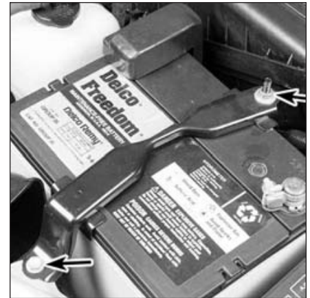
9.8 Make sure the battery clamp nut and bolt (arrows) are tight
